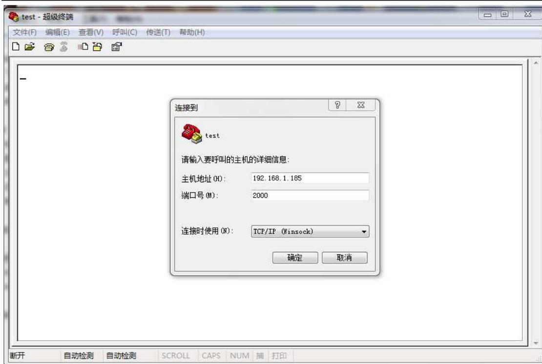
When it connected with your WIFI shield. You should see the response `*HELLO*`. Green LED D1 state on solid. Settings to allow you to see what you are typing in Hyperterminal once connected to the WiFi shield you should be able to send data to Arduino through WiFi. Just input data into Hyperterminal input blank, and the serial monitor of arduino which connected with arduino will show the data arduino receives.
